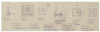
The sequence of transformations that gets object from its original object space into screen space.
